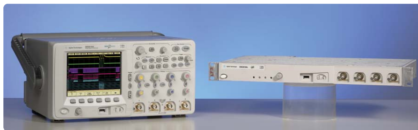
Figure 6. The 6000A and 6000L Series oscilloscopes are 100% software compatible, enabling smooth test system transition.
