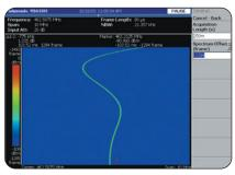
RSA Series Spectrogram uniquely shows time-varying signal behavior in frequency change/stability, spectrum occupancy, pulsed signal timing, power change and more! The sample above shows the frequency settling characteristic of a transmitting device.
