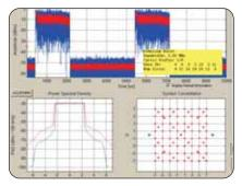
The RSA3408B is your best tool for both troubleshooting and conformance testing. Here, a mobile WiMax analysis is performed using RSA-IQWIMAX software.
