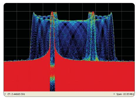
Revolutionary DPX spectrum display reveals transient signal behavior that helps you discover instability, glitches and interference. Here, an infrequently occurring transient is seen in detail. The frequency of occurrence is color-graded, indicating the infrequent transient event in blue and the noise back-ground in red.
