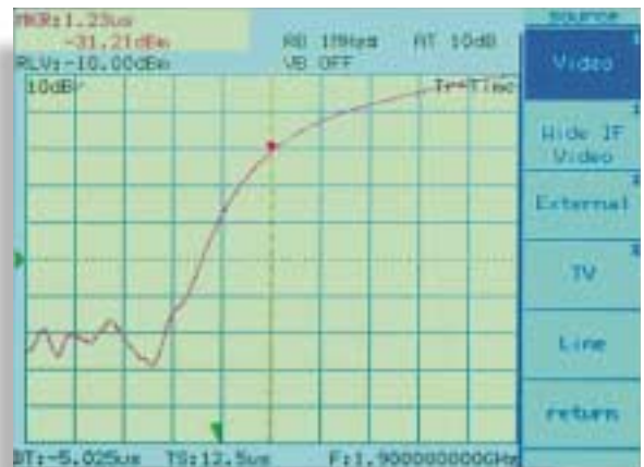
High-speed time-domain measurement (TS=12.5 \mu s)
