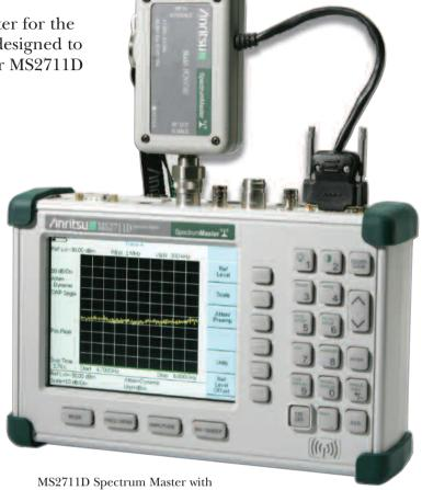
MS2711D Spectrum Master with FCN4760 block down converter
