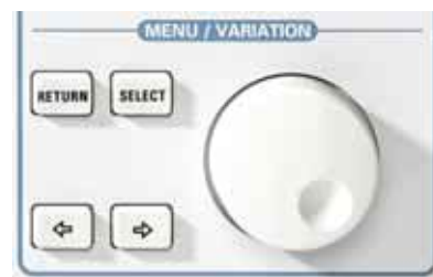
FIG 10: General settings and menu selection with spinwheel, RETURN, SELECT and arrow keys
