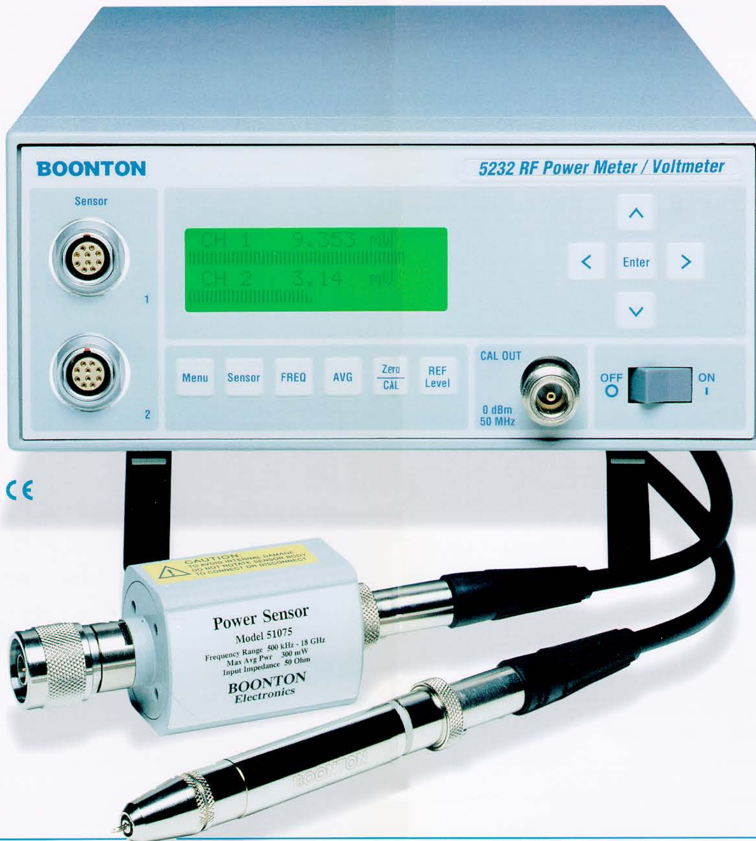
High-speed readings offer a new level of precision testing. With advanced digital signal processing and fast-response sensors, Boonton's 4230A and 5230 series provide > 200 readings per second over a 90-dB dynamic range for fast, accurate testing and increased manufacturing throughput.
