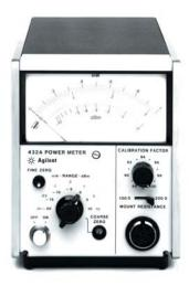
As today's power measurements become more complex, it is increasingly difficult to make reliable, accurate power measurements. For more than 40 years, you've depended on Agilent's 432A analog power meter, used with temperature compensated thermistor sensors to provide high accuracy over a wide temperature range.
