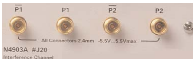
Figure 15: Interference channel connectors
