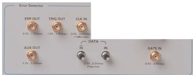
Figure 13: Front panel connectors for error detector
