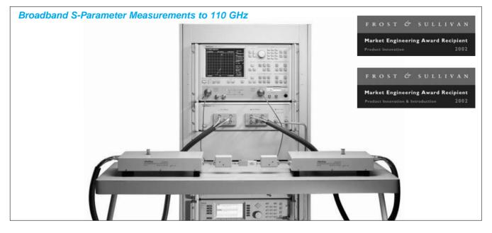
The ME7808A Broadband Vector Network Analyzer (VNA) is a high performance measurement solution that covers 40 MHz to 110 GHz in a single fast sweep. In contrast to the millimeter wave Vector Network Analyzer, the ME7808A is built on the advanced technology of the Lightning 65 GHz VNA, and extends its advanced features and intuitive user interface to 110 GHz.
